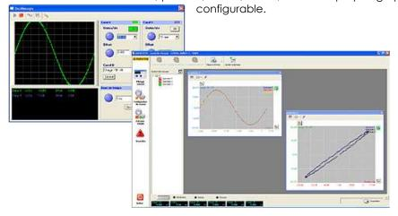
All the defined channels, including direct values from transducers, calculated channels, external channels, time, can be recorded by means of the data acquisition software included. Different acquisition modes, sample rate, start/stop conditions, storage addressing, etc are available in SCM4000.
