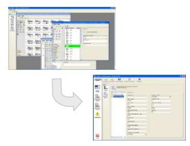
The SCM4000 Control Panel Module is also used to display in real time the quantities involved in the test and the results from the recorded data: cycle number, the total stress range, the mean stress, the elastic, plastic and total strain ranges, the raising and falling moduli and the hysteresis loop area for each captured loop is incorporated into the software package.
