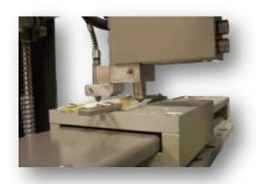
Scratch test will be able to push the cover to the limit into a progressive load test, or submit it to successive scratch cycles simulating a fatigue test or, on the other hand, characterize its scratch hardness measuring with the optical microscope the resultant groove's width.
