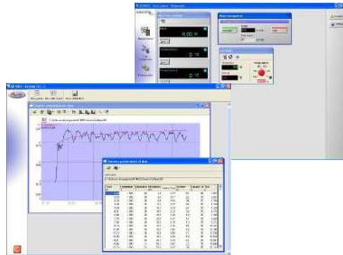
Selection of the control commands: frequency, number of cycles, etc. The preset timer built in software stops the machine after a set time. Actually, tests can be defined up to more than 500h. For this purpose, the proposed system includes an uninterruptible power source for the whole tribometer and computer.
