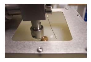
The heater block is mounted on flexures, which are stiff in the vertical (loading) direction, but offer limited resistance to horizontal forces. This system is used as a linear flexure bearing for frictionless horizontal guiding. Movement in the horizontal direction is restricted by an additional 500N KISTLER 9217A piezo-electric
